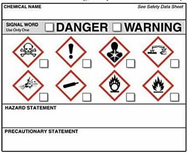
The GHS system utilizes 6 elements to communicate the hazard associated with the chemical the label is associated with.
